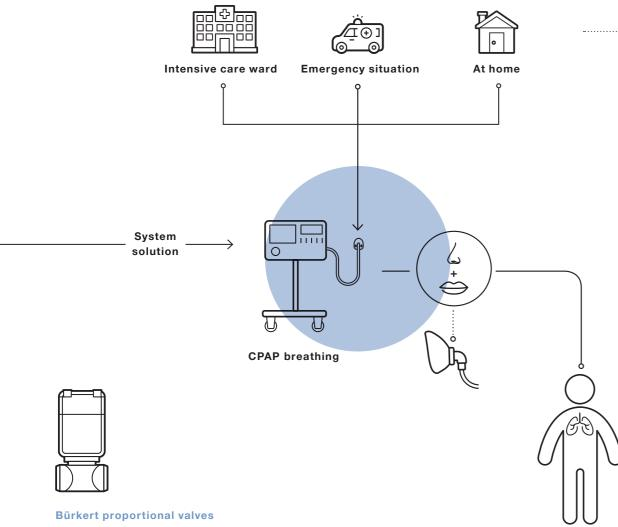
operate without friction, with short response times and a repeat accuracy of ± 0.25%. This allows you to achieve a significantly lower deviation from the set value in the volume flow of the gas mixture than the legally required  $\Delta Q \leq \pm 2\%$  at 20 litres per minute.
