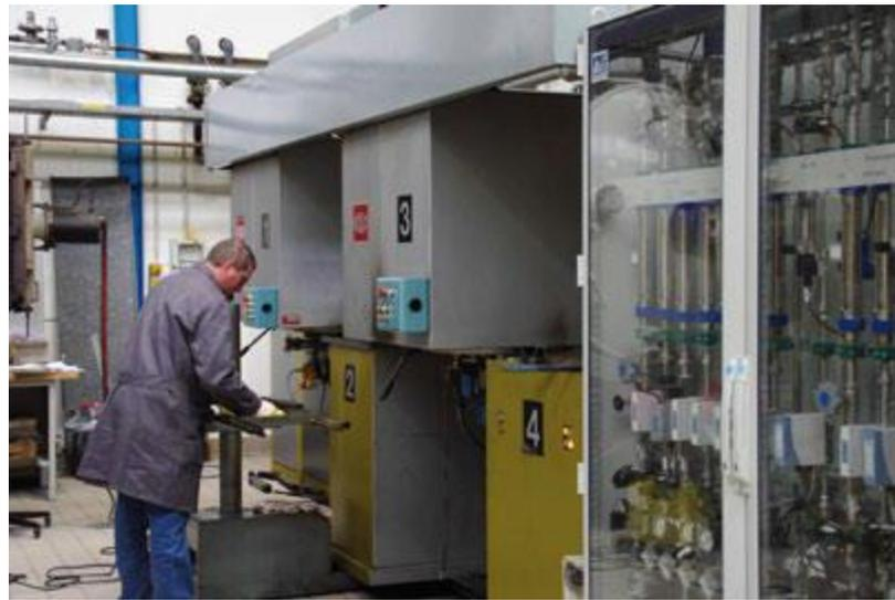
Fig. 1: Furnace for heat treatment using various processes at the foundation Institut für Werkstofftechnik (IWT) in Bremen
